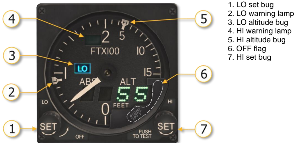
Figure 5.4. AN/APN-209 radar altimeter
