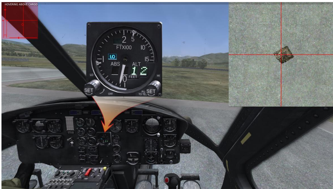
Figure 11.7. Conditions for Automatic Attachment of Load at Hovering Method (1 of 2).
