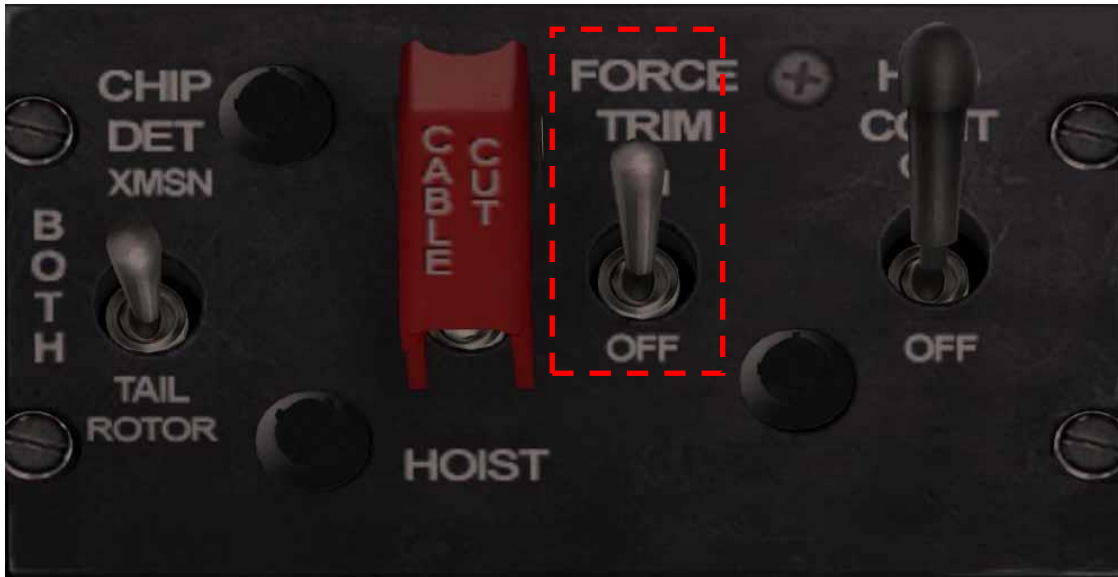
Figure 4.8. FORCE TRIM ON/OFF switch.
