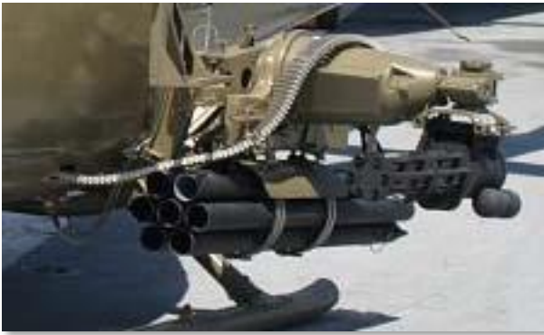
Figure 8.2. Elements of M21 Subsystem Assembly on the Left Side of the UH-1H.
