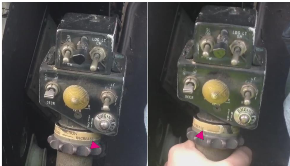
Figure 9.1. Direction of Rotation of the Throttle.
